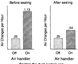
Sealing the duct system can dramatically decrease house infiltration.
