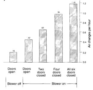
Closing interior doors can significantly increase air infiltration.
