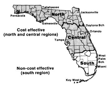
In North and Central Florida heat pumps are a cost-effective choice for electric space heating. There are two main types of heat pumps, air-toair and ground-source. Both operate on the same principle but use different cooling and heating sources.
