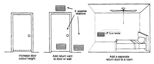
Provide adequate air return capacity for when doors are closed.
