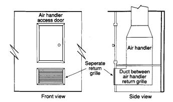
Use a solid door for air handler access and a separate sealed return duct from the air handler to a grille below.
