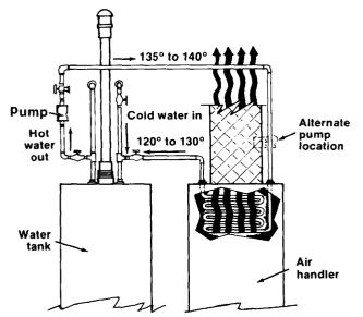
Forced-air hydronic systems use hot water to supply heat.
