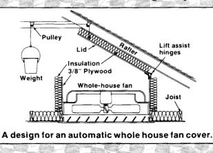
was assembled in the attic, he attached two pulleys to the rafters with screw eyes, then added to a weight bag until the force of the whole-house fan lifted the insulated box lid easily.
