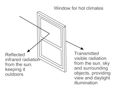
The visible transmittance of glass is the fraction of incident light transmitted by the glass to the It has the interior. symbol VT (or  $T_{y}$ ) in window product literature, and is a number ranging from 0% to 100% (or 0 to 1.0 in fractional terms). "Spectral selectivity," denotes the ability of a glass (or its coating) to transmit radiation variably over the spectrum-it might be high over the visible portion and low over the infrared portion. In this way it transmits radiation
