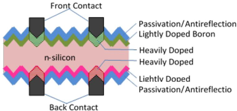
Figure 3: Bifacial Silicon Solar Cell.
